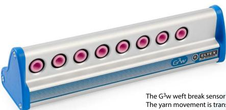
The G<sup>3</sup>w weft break sensor operates on the piezoelectric principle. The yarn movement is transferred into an electric signal, which is amplified and evaluated within the sensor. The weft sensor has a current logic output and is manufactured with 4 or 8 eyelets.
